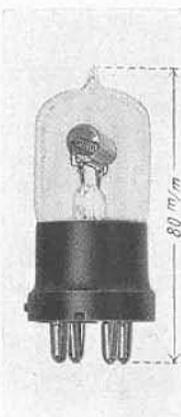
For small amplifiers, audion receivers, interference transmitters and H. F. amplifiers, with iron resistance. / Heating current 0,53 to 0,56 amps. Anode voltage from 45 to 90 volts.
