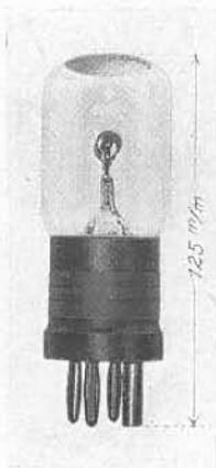
For low frequency amplifiers, audion receivers, interference transmitters and H.F. amplifiers; with iron resistance. heating current 0,53 to 0,56 amps., anode voltage 45 to 90 volts.
