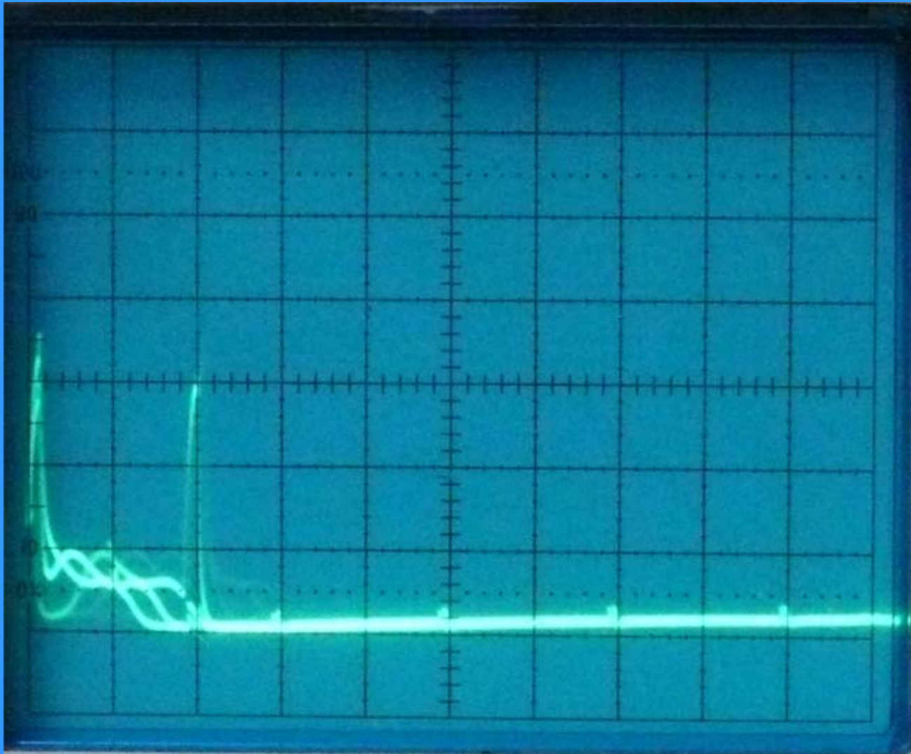
Watching the FuG 25a signal output at pin 9 of the test connector
