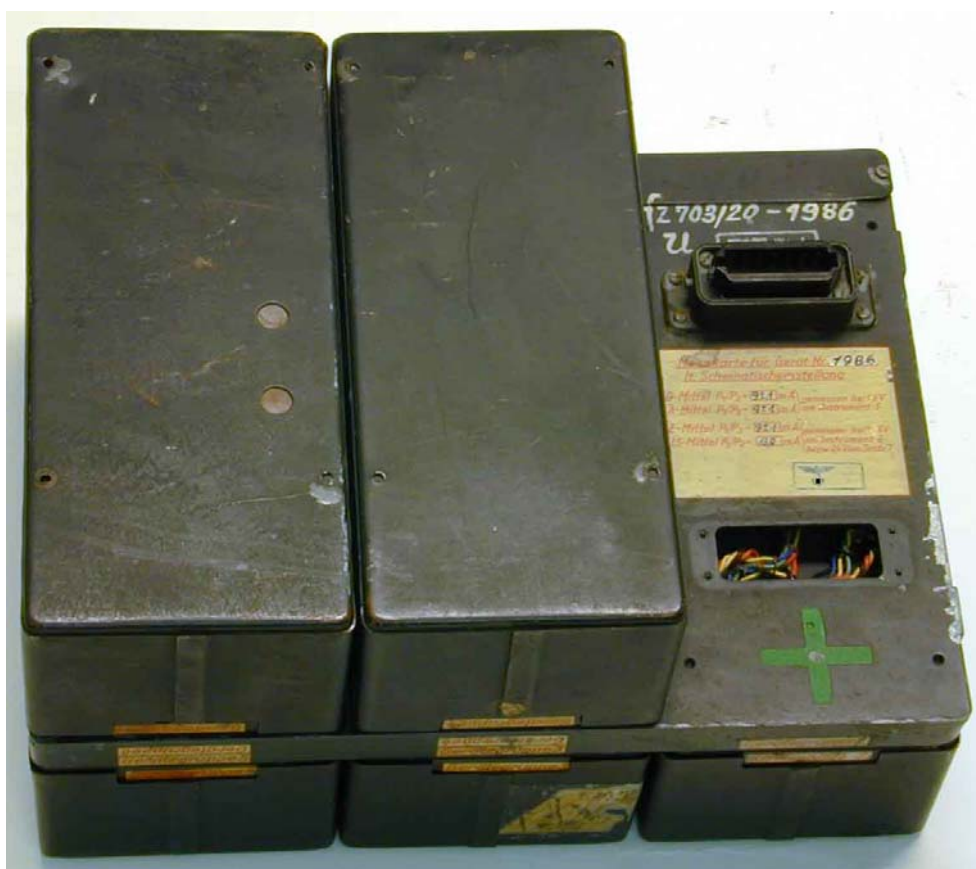
Photo 1: Shown here is the final version of Hoelzer's analog computer called: Mischgerät. It consists of 5 modules (two in front and 3 mounted on the other side of the central chassis).
