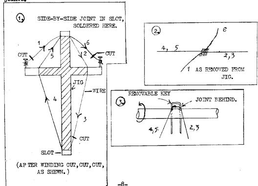
The wire and joint were then placed on a straight mandrel with a central removable key and the springs were formed by rotating the mandrel. The key is afterwards removed in order to withdraw from the mandrel.
