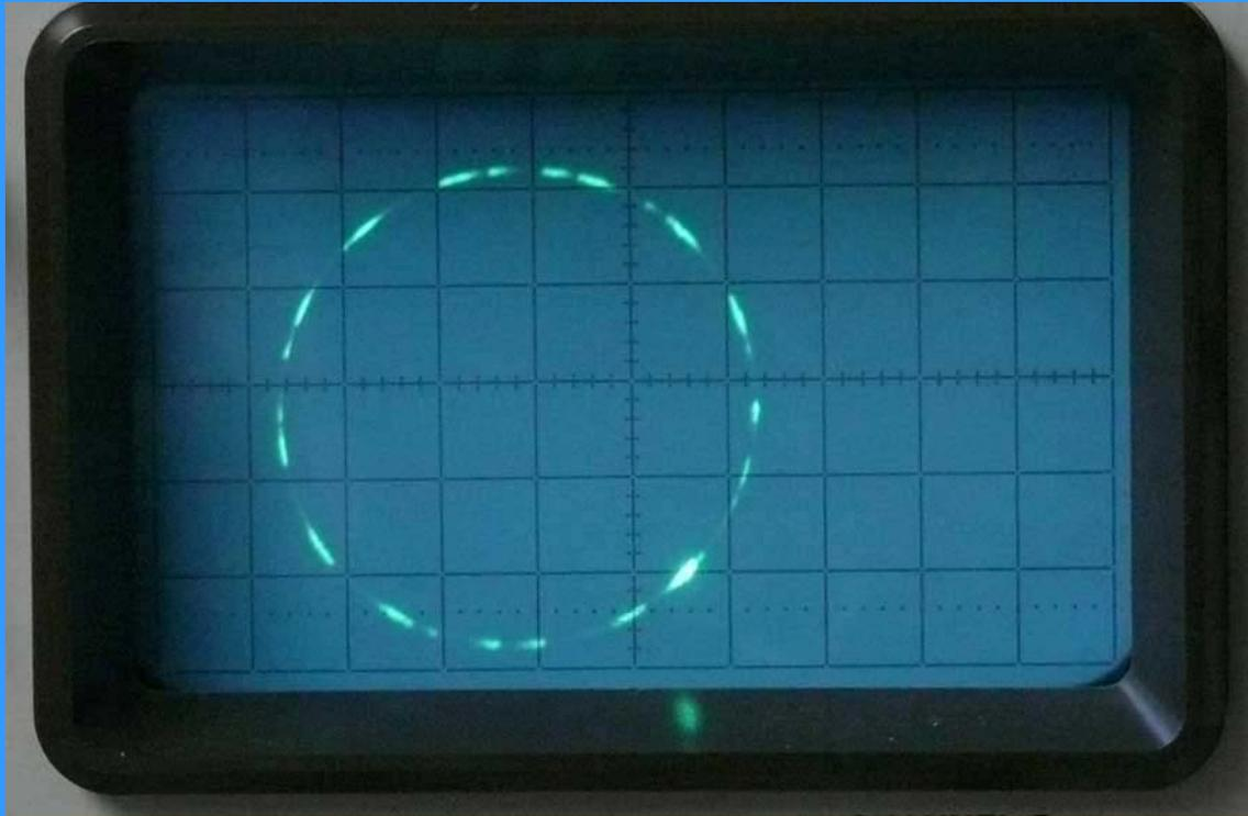
The a bit brighter spot is an example of an 'order' signal, painted at a simulated aircraft display; using a Lissajous. The dashes originate from the also available EGON pulses, though having a lower PRF (500 versus 506 Hz). These do not interfere with the actual Nachtfee data content. But is part of the combined EGON/Nachtfee signals
