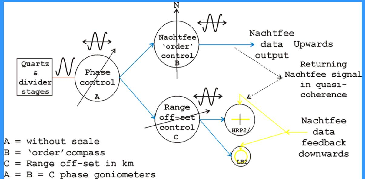
Firstly, the pulse due North is correctly adjusted by means of goniometer C
