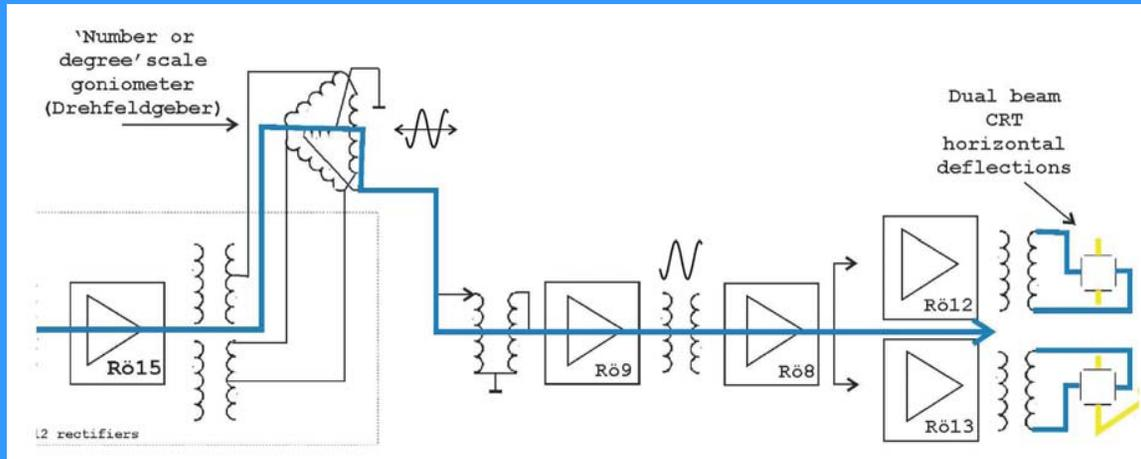
Due north on the left is the Nachtfée feedback pulse adjusted back-to-back in the centre of the dual trace CRT correctly; by means of the number or 'Range off-set' control. Using the goniometer on the left-hand side
