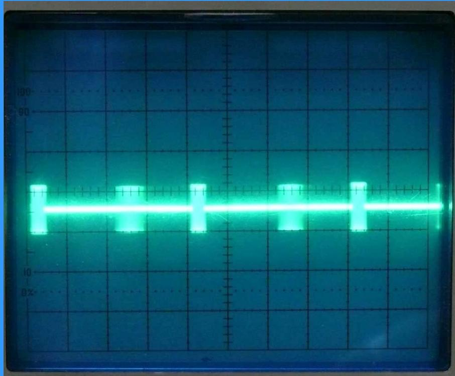
Viewing the combined HF signals send towards the simulated aircraft system
