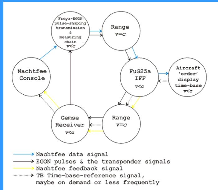
The Nachtfee data pulse has got a data or 'order' phase off-set in such a way that it will arrive at the aircraft display in accordance to the actual Nachtfee compass pointer.
