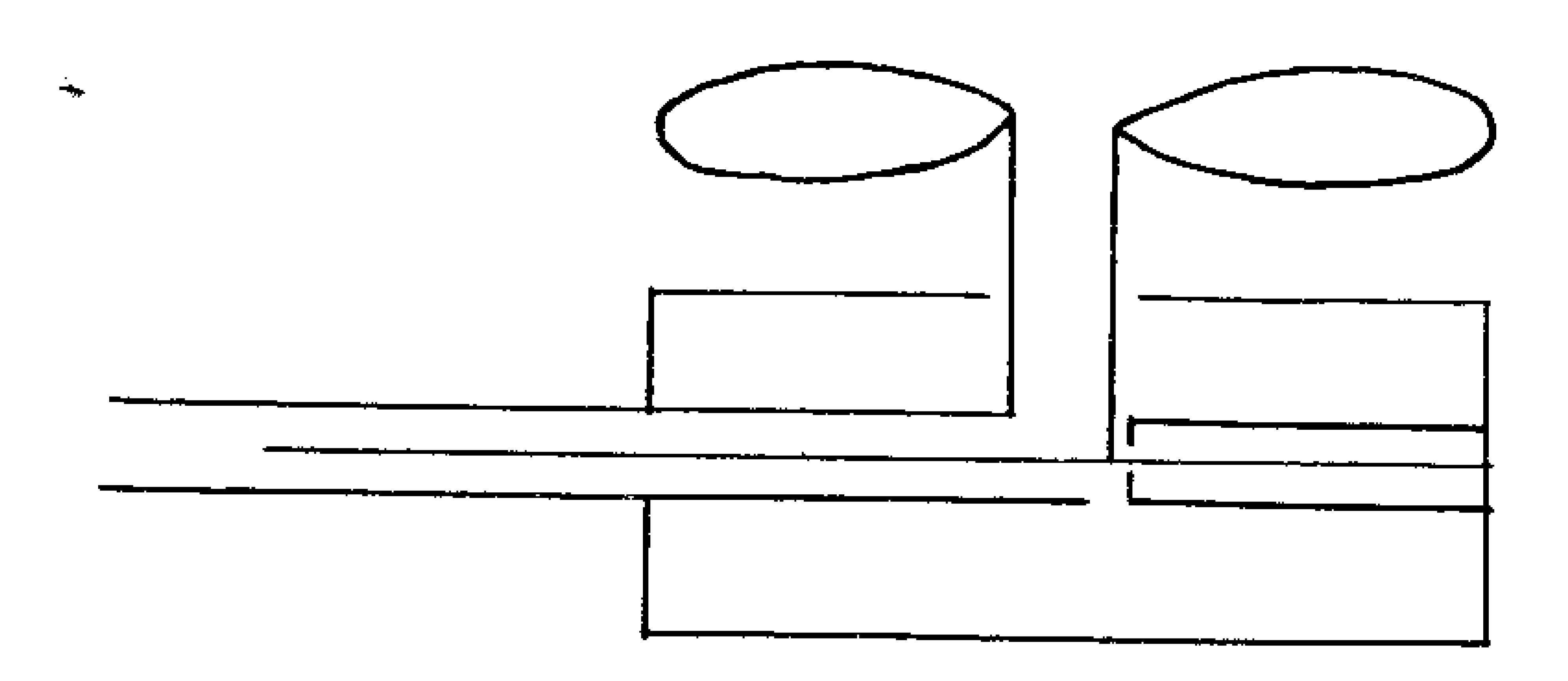
4.4. Broad-band concentric cable matching transformers of two types had been developed, the first type consisting of a constant diameter inner conductor and an exponentially tapered outer conductor, and the second type having a constant diameter outer and an exponentially tapered inner conductor. The cables were capable of matching from 200 - 600 ohms.
