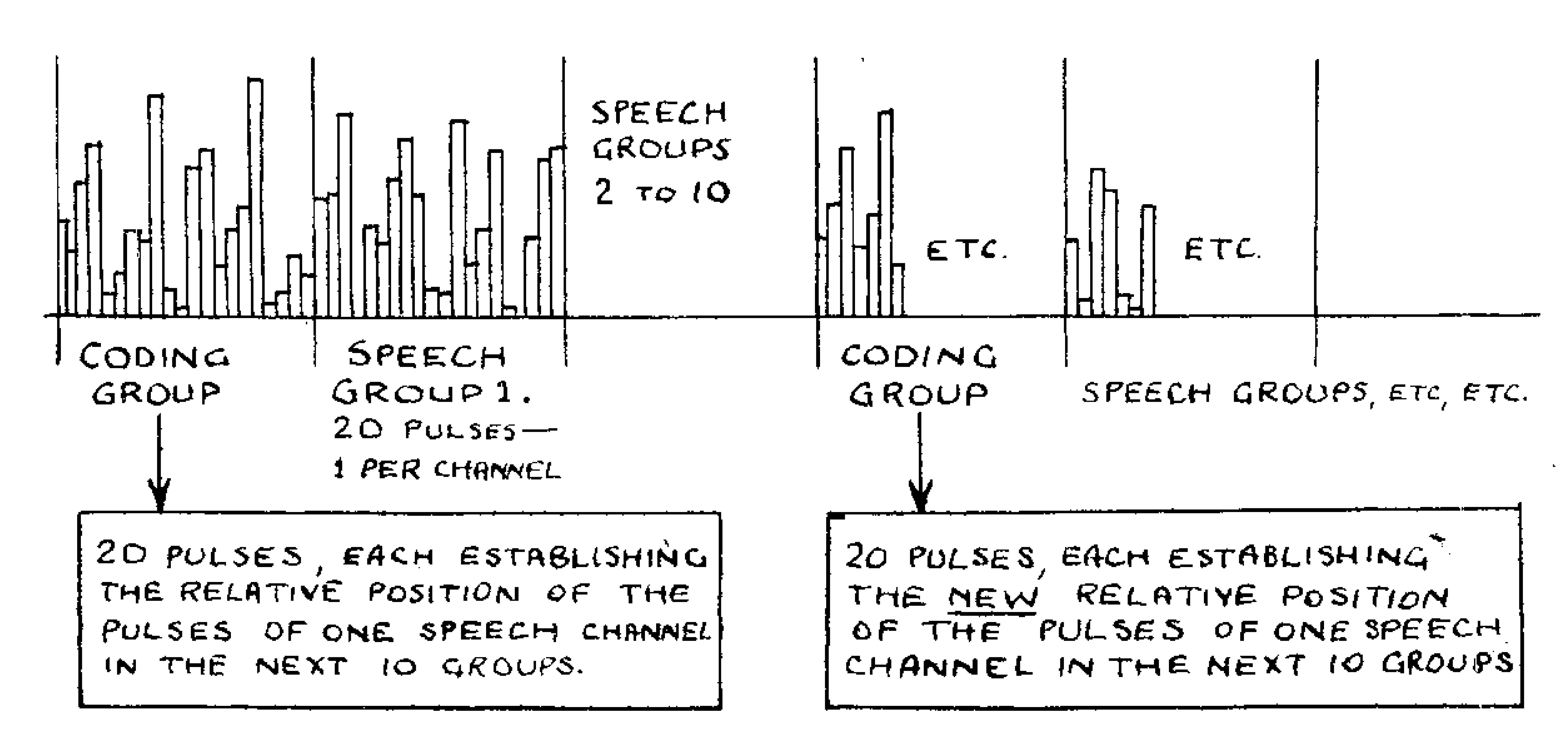
FIG. 2 TYPICAL ARRANGEMENT OF CHANNEL PULSES
