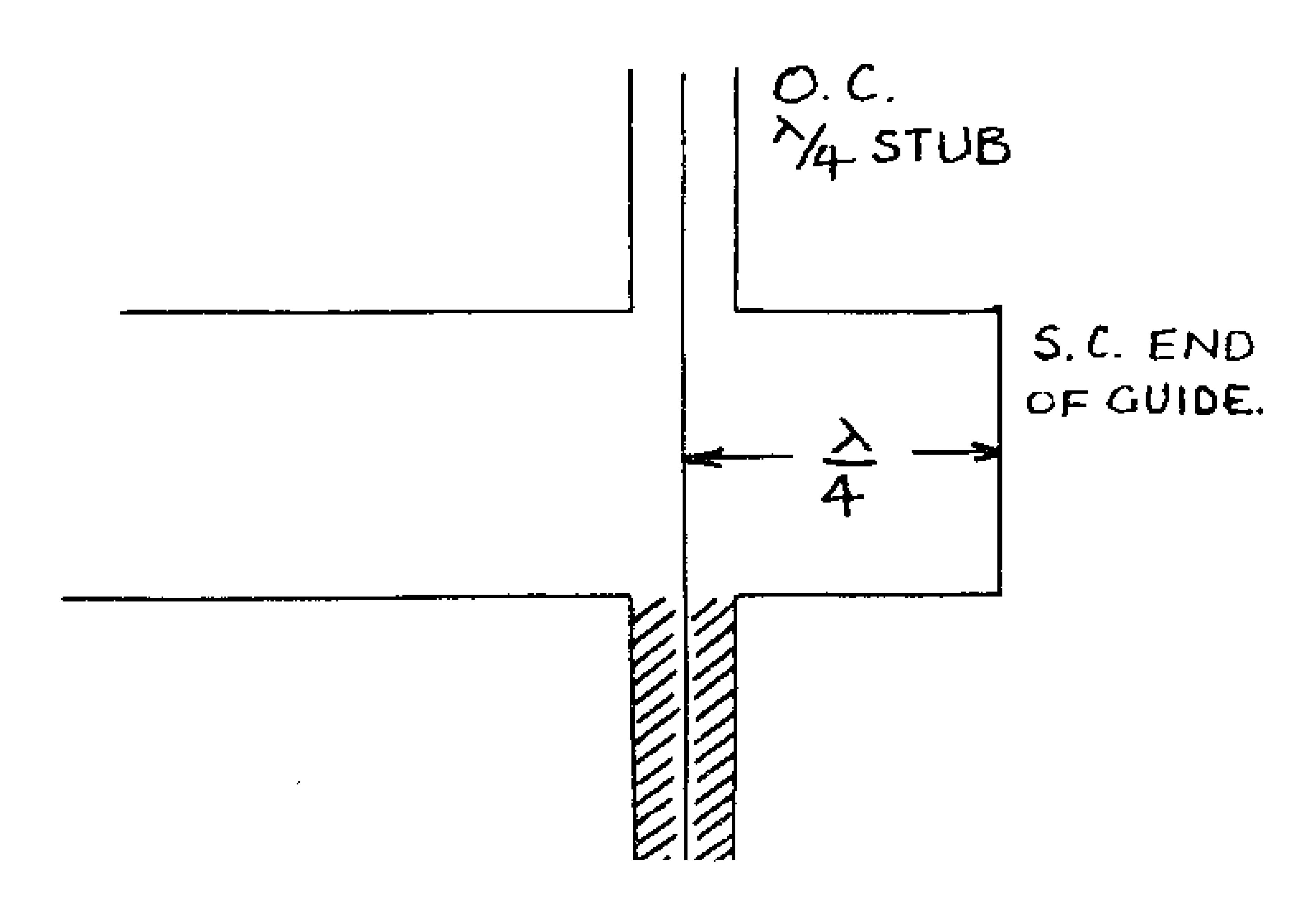
The above arrangement was used for a range of wavelength of 1 to 2 cms.
